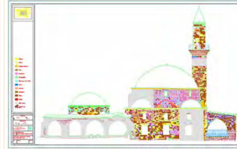
Stone Visual Deterioration Maps
